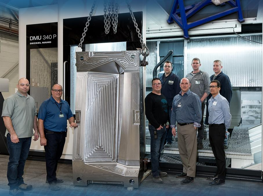
**Nickel Vapor Deposition capability has led us to be the leading supplier for shell tooling with integrated heating. Ideal for Out of Autoclave, Rotational Molding or Vacuum Infusion.**
