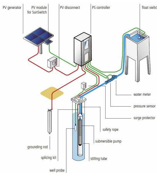
The benefit of a solar powered system is the low installation cost compared to the cost of running mains power to a site, or purchasing and running a generator. The running and maintenance costs associated with a solar powered pump is low even compared to a windmill type pump.
