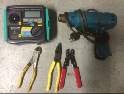
Tools required to cut, crimp, heat and test completed cable splice.
